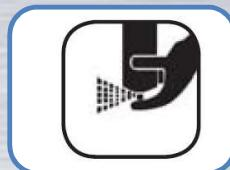
The spray nozzle can stick. This can be avoided by holding can upside down and briefly emptying the nozzle and valve when you are finished.
